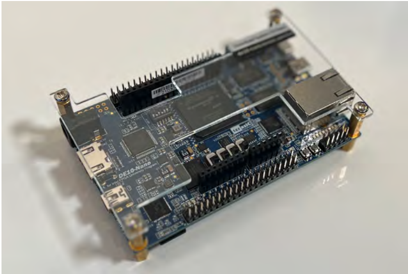
Fig. 5. DE10-Nano FPGA Platform used in the MiSTer Project. MiSTer, first introduced in 2017, is a rapidly developing open-source project that is used to emulate multiple platforms, most commonly for video game software. (Image Credit: Andrew Borman)
